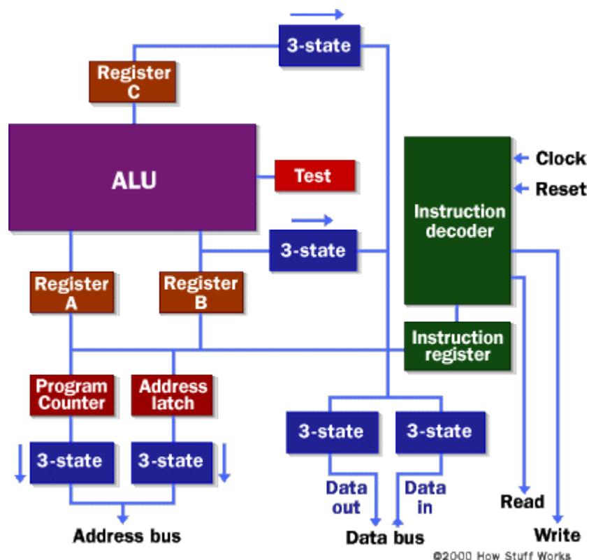
This is about as simple as a microprocessor gets. This microprocessor has:
